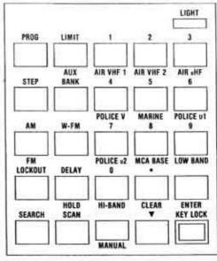
Step: The step key allows you to choose a frequency step in the range from 5 KHz to 995 KHz or any multiple of 12.5 KHz. This function may be used in Manual, Scan or Search modes.
